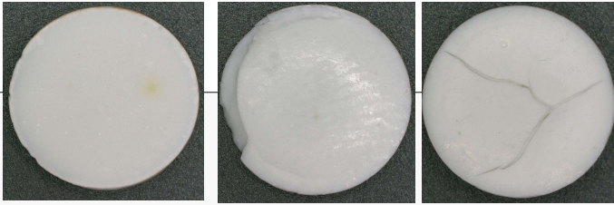
Figure 1. A representative set of 5% Zn discs showing variations in disk surface morphology, including chips, divots, and cracks imaged at 50x magnification using a light microscope.
